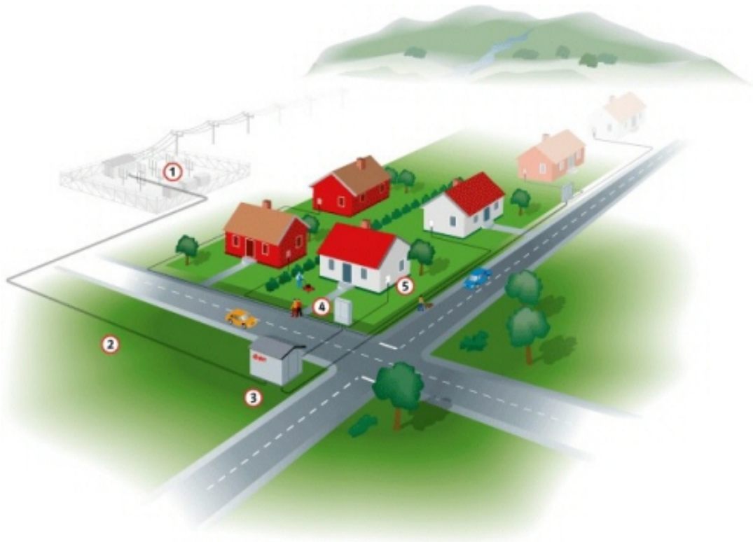
Figure 2.2: Grid structure in residential area. 1: Distribution station, 2: High voltage cable, 3: Transformer station, 4: Cable cabinet, 5: Connection to house, [11]
